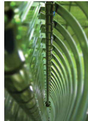
The 3 MV Electrostatic Accelerator (above) is the largest dust accelerator in the world and is available for use by the lunar, space and plasma physics communities. Photo © Keith Drake.
